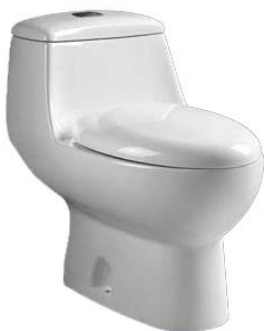
Model: ZS1278 One-piece toilet (Siphon) Size: 705x420x640mm S-trap: 300mm Roughing-in
