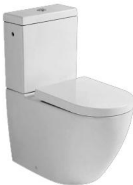
Model: AS1932 Two-piece toilet (Washdown) Size: 680x375x810mm S-trap: 250mm Roughing-in P-trap: 180mm Roughing-in
