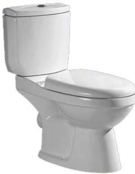
Model: AS1233 Two-piece toilet (Washdown) Size: 680x385x745mm S-trap: 250mm Roughing-in P-trap: 180mm Roughing-in
