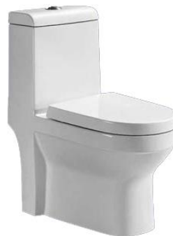
Model: ZS1604 One-piece toilet (Washdown) Size: 690x350x805mm S-trap: 250/300mm Roughing-in P-trap: 180mm Roughing-in
