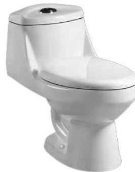
Model: ZS1409 One-piece toilet (Siphon) Size: 735x385x680mm S-trap: 300mm Roughing-in
