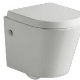
Model: MS2304 Wall-hung toilet (Washdown) Size: 480x365x360mm P-trap: 180mm Roughing-in
