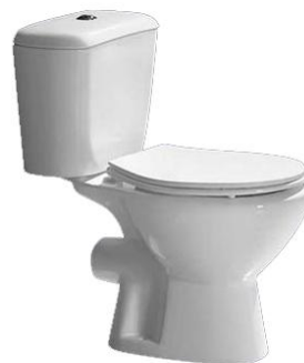
Model: AS1209 Two-piece toilet (Washdown) Size: 650x370x725mm S-trap: 250mm Roughing-in P-trap: 180mm Roughing-in
