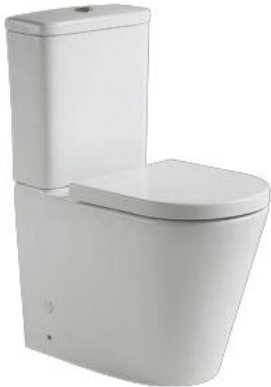
Model: AS1304 Two-piece toilet (Washdown) Size: 642x380x850mm S-trap: 250mm Roughing-in P-trap: 180mm Roughing-in
