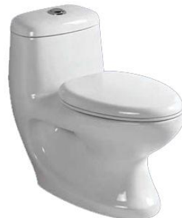
Model: ZS1751 One-piece toilet (Washdown) Size: 710x390x650mm S-trap: 250/300mm Roughing-in P-trap: 180mm Roughing-in
