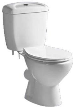
Model: AS1983 Two-piece toilet (Washdown) Size: 675x360x760mm S-trap: 250mm Roughing-in P-trap: 180mm Roughing-in
