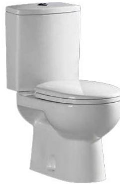
Model: AS1073 Two-piece toilet (Washdown) Size: 650x355x760mm S-trap: 250mm Roughing-in P-trap: 180mm Roughing-in
