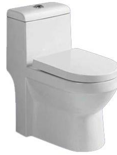
Model: ZS2604 One-piece toilet (Washdown) Size: 630x340x705mm P-trap: 180mm Roughing-in S-trap: 250/300mm Roughing-in
