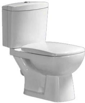
Model: AS1329 Two-piece toilet (Washdown) Size: 690x390x740mm S-trap: 250mm Roughing-in P-trap: 180mm Roughing-in
