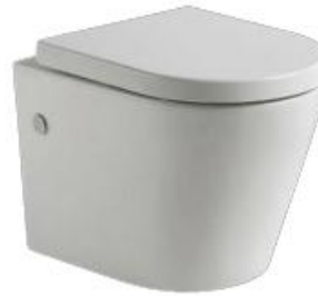
Model: MS1304 Wall-hung toilet (Washdown) Size: 480x365x360mm P-trap: 180mm Roughing-in
