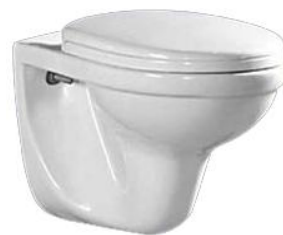
Model: MS1176 Wall-hung toilet (Washdown) Size: 535x340x370mm P-trap: 180mm Roughing-in
