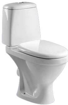
Model: AS1119 Two-piece toilet (Washdown) Size: 650x330x740mm S-trap: 250mm Roughing-in P-trap: 180mm Roughing-in
