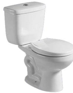
Model: AS1210 Two-piece toilet (Siphon) Size: 680x425x745mm S-trap: 300/400mm Roughing-in
