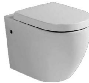
Model: MS1932 Wall-hung toilet (Washdown) Size: 550x365x380mm P-trap: 180mm Roughing-in
