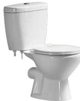
Model: AS1168 Two-piece toilet (Washdown) Size: 675x385x760mm S-trap: 250mm Roughing-in P-trap: 180mm Roughing-in
