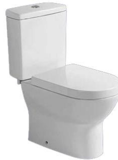
Model: AS1958 Two-piece toilet (Washdown) Size: 700x380x790mm S-trap: 250/300mm Roughing-in P-trap: 180mm Roughing-in
