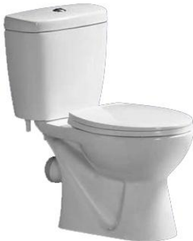
Model: AS1105 Two-piece toilet (Washdown) Size: 695x385x750mm S-trap: 250mm Roughing-in P-trap: 180mm Roughing-in
