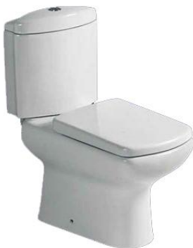
Model: AS1951 Two-piece toilet (Washdown) Size: 660x405x785mm S-trap: 250mm Roughing-in P-trap: 180mm Roughing-in
