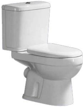
Model: AS1306 Two-piece toilet (Washdown) Size: 690x410x765mm S-trap: 250mm Roughing-in P-trap: 180mm Roughing-in
