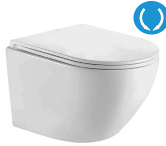
Model: M3370B Wall hung toilet (Rimless) Pan size: 515X360X380mm P-trap: 180mm Roughing-in
